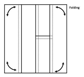
Figure 2: Folded EPDM membrane in the wall corners
