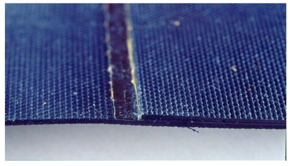
Figure 6: Cross-section of a joint of the sheet
