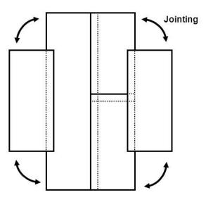
Figure 1: Wall corner joints according to FLL method
