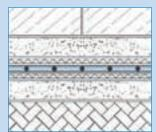
**NOVOPROOF® TE** as sealing sheet in a retardation basin Composite masonry
